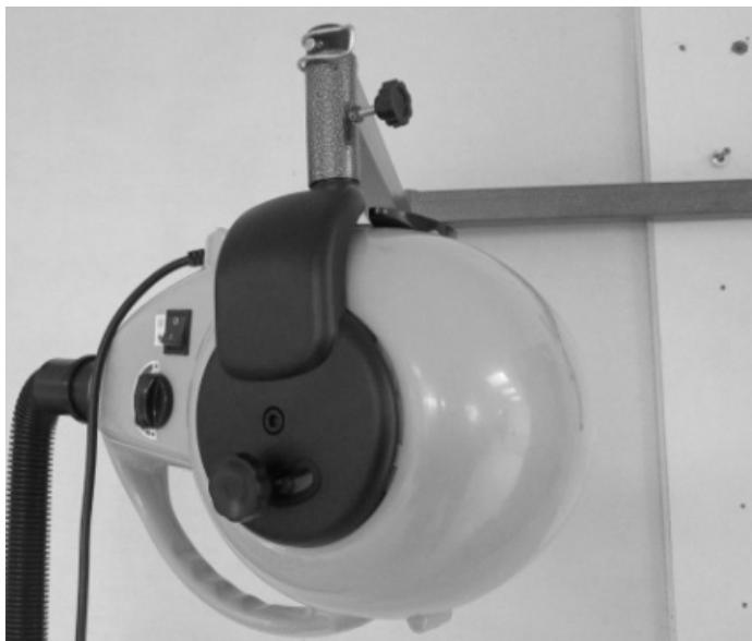
Then place the adjustment wheel on the side to allow inclination of the dryer-blaster. (non-contractual pictures)
